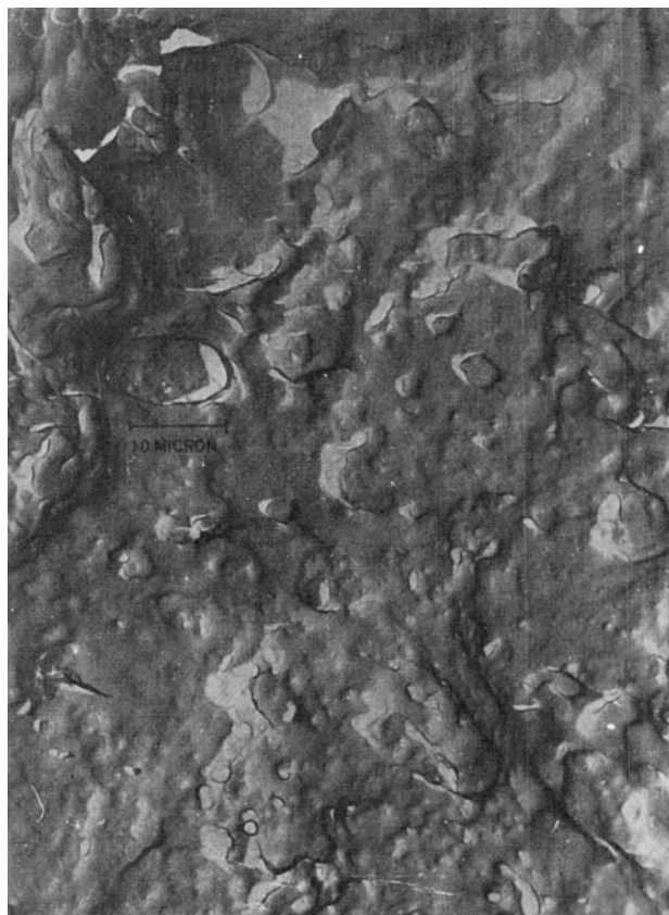
Fig. 7. A typical electron micrograph of the copper heater surface.
